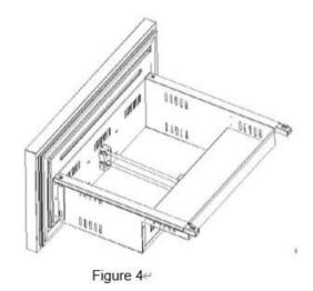
**Étape 5:** Install S.S. tube to prevent bottles placed in the lower drawer from falling during opening and closing the door.
