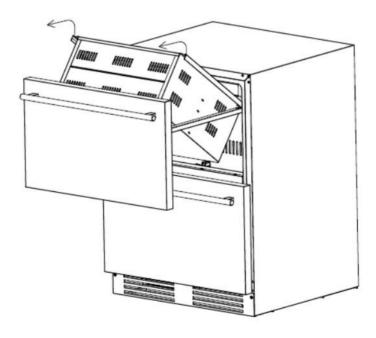
3. To remove it, turn the charcoal filter to set free pins and pull it directly from the inside of the cellar towards you
