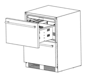
2. Grab the sides of the drawer and lift the drawer up at 45 degrees, and then remove out the drawer
